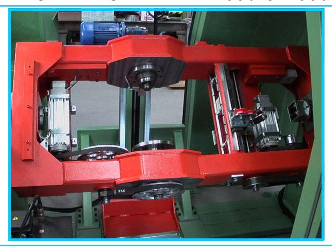
Suitable for the laying up of delicate products such as optical fibres cables, screened cables glass or copper braided, P.T.F.E. insulated cables.
